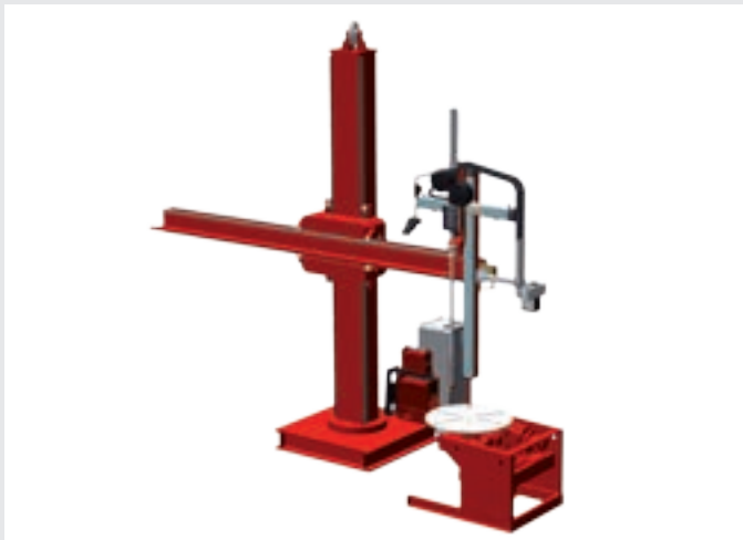
/ Conventional Cladding System
