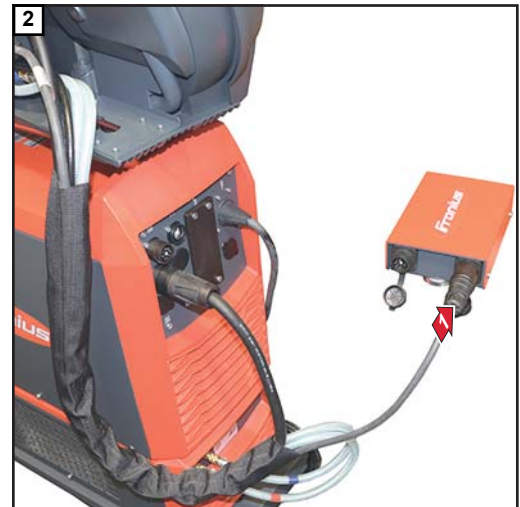
Connect the SpeedNet cable from the interconnecting hosepack to the SpeedNet distributor box
